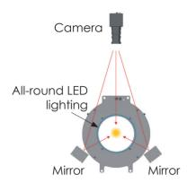
Thanks to a mirror system and a very powerful all-round lighting that eliminates shadows, **every vegetable is subjected to a perfect 360° analysis.** The optical system generates 3 immaculate high-resolution images of each carrot. These can be displayed immediately on the computer screen to check the error detection.
