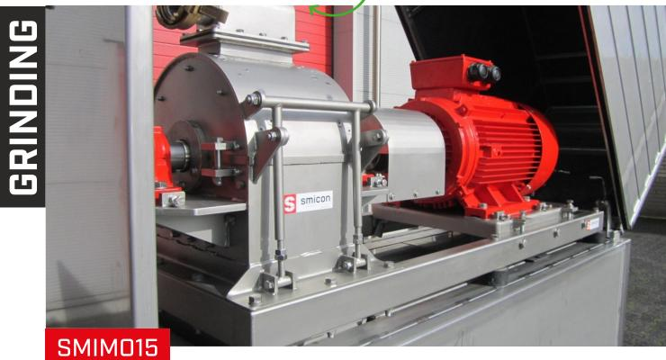
The rotor inside the SMIMO grinder pulverizes organic products into a homogeneous pulp which is suitable for pumping. A sieve inside the grinder ensures that the product is only discharged once the particles have the required size. The noise level can be reduced by an acoustic cover (if necessary). Parts can be easily exchanged and the grinder is very resistant to aggressive products and substances.
