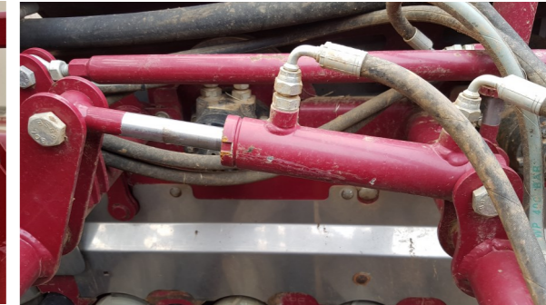
Standard clod roller height control: turnbuckle (In store) or hydraulic ram (mobile version). All clod rollers are linked and raise/ lower together (8 row version is split 4 + 4).
