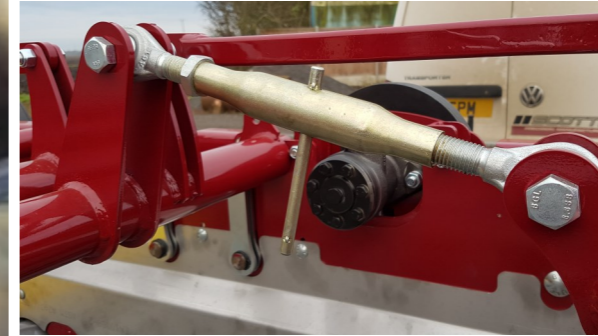
Standard clod roller height control: turnbuckle (In store) or hydraulic ram (mobile version). All clod rollers are linked and raise/ lower together (8 row version is split 4 + 4).
