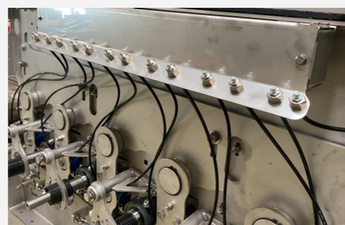
Remote greasing kit fitted as standard for all bearings (In store and mobile version)
