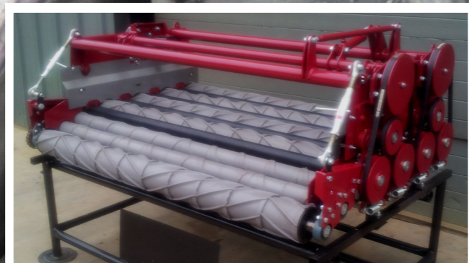
Mobile: hydraulic drive with Kevlar V belts
